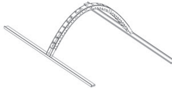
1. CENTRAL ROW OF CRATES AND ADJACENT RIBS ASSEMBLED ON GROUND AND TITLED UP INTO PLACE
