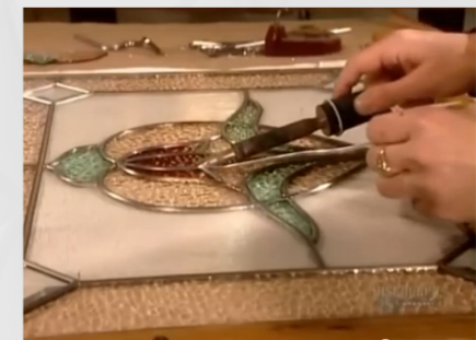
Solder every joint of lead
